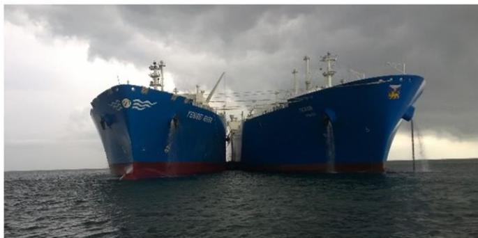
*LNG transfer from Pskov gas carrier to Yenisei LNG tanker*
